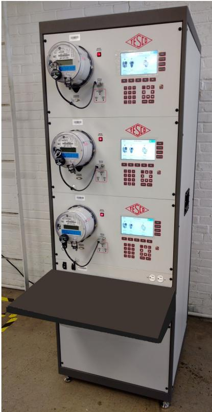
Perform qualification, disconnect, communication, and advanced functional tests with TESCO's new **Meter Engineering Board**. With basic metrology (0.1% accuracy) TESCO's new MEB can also be used as a demand board or a time run board, as part of meter certification, or to meet regulatory testing requirements. A new socket design provides automated operation to make loading easier. All new TESCO boards include our new electronically actuated sockets.
