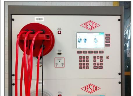
TESCO's Calibration Adapter (Cat. 2450) is a socket adapter designed to bring phase A, B, and C current and potentials of a TESCO multi-position test board to an external reference standard for calibration of the test board.
