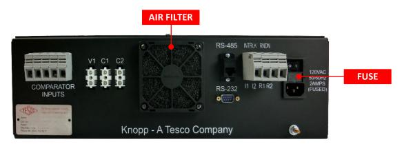
Figure 5.2. KATC-V2 Fuse and Air Filter location
